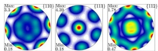
**Figure 1.** Simulated pole figure for the surface at 300 °C Rolling.
