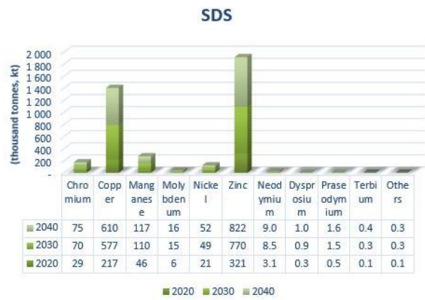
Figure 2. SDS scenario: the assessment of mineral materials and also rare-earth elements required for the wind energy industry in the coming years.
