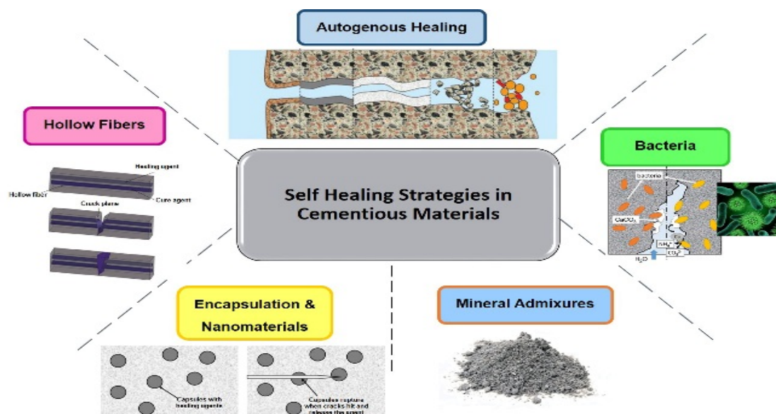
Figure 1. Schematic diagram of self-healing strategies in cementitious materials
